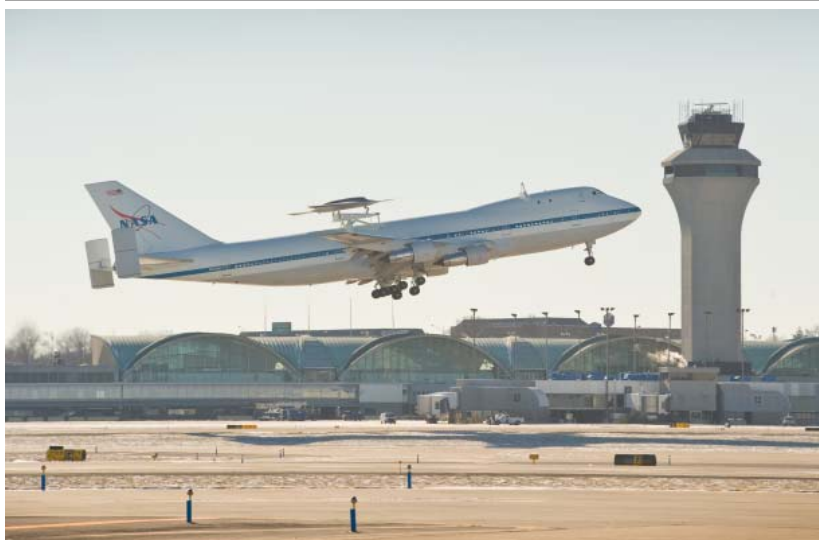
The Phantom Ray in the saddle atop a 747 for a test flight.
