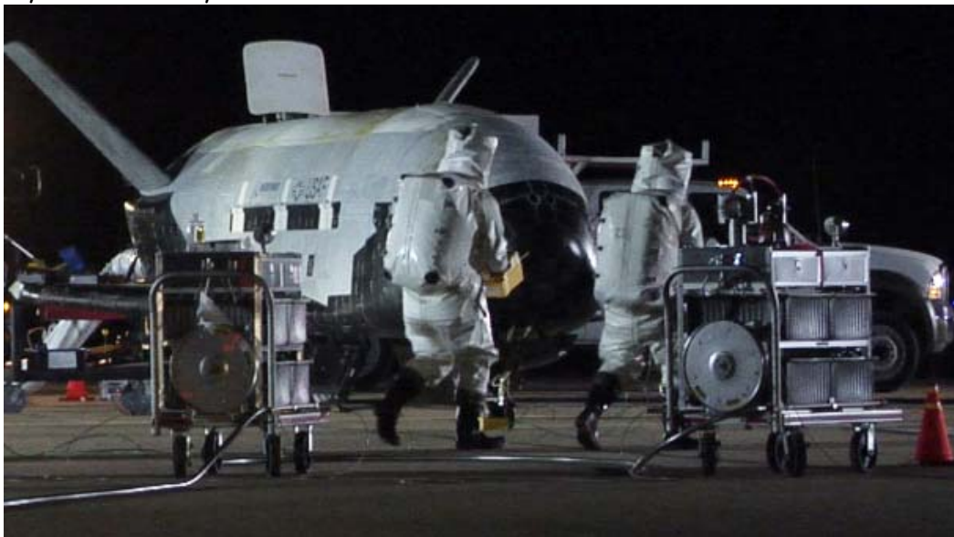
Air Force personnel in "self-contained atmospheric protective ensemble suits" perform initial post-orbit checks on the X-37B space plane early today on a runway at Vandenberg Air Force Base.
